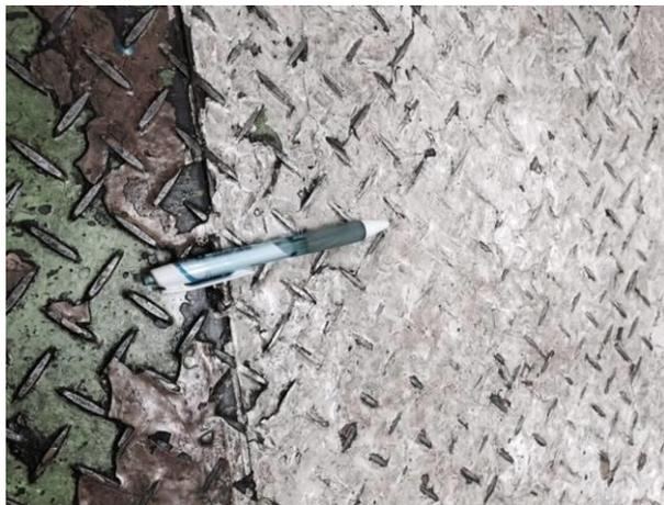
To paint on carbon steel checker plate for refurbishment bridges the gap that exists between dots and makes it slippery.
